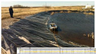
Determining the amount of sediment in a tailings pond is achieved while using an unmanned boat and GPS enabled data acquisition. A 250 MHz antenna achieves 1.5 metres of high resolution imagery, as seen below.
